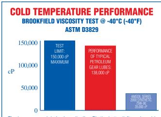
The lower a gear lube's viscosity (in cP), the better it flows in cold temperatures. AMSOIL Series 2000 Synthetic 75W-90 Gear Lube significantly outperforms conventional petroleum lubes, which means it offers significantly better protection against wear.
